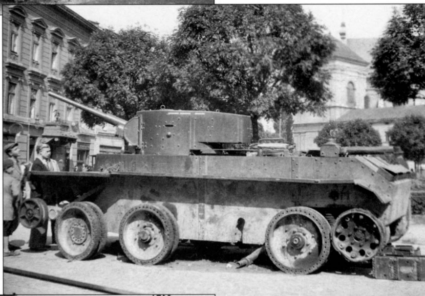
A damaged BT-7 tank sits abandoned on a street in Lvov. Note the three small horizontal white bars on the top part of the side of the turret — they are remainders of the full marking system used in the 1930s. The white dotted line indicates the 2nd company.
