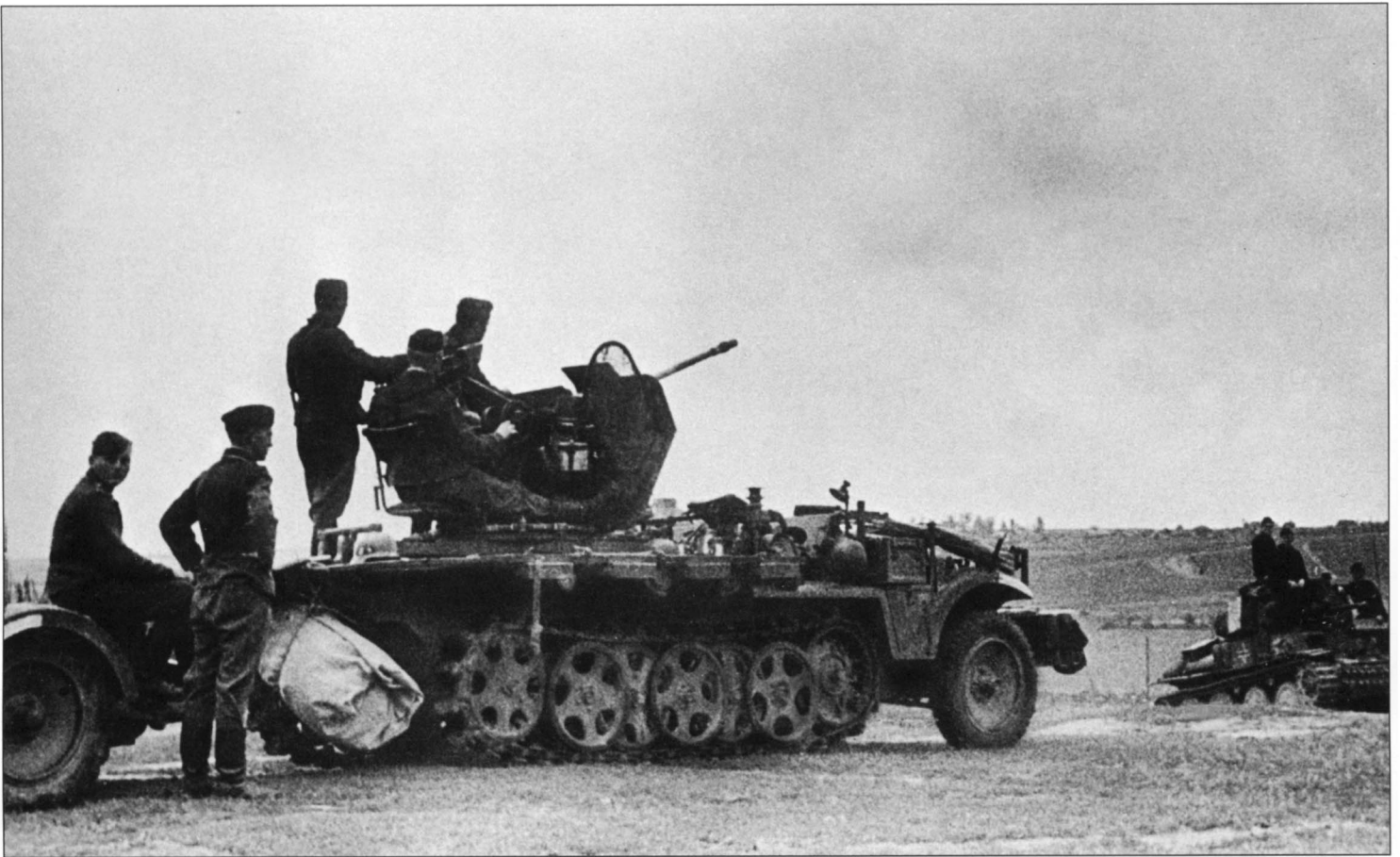
The crew of a Sd.Kfz. 10/4 is ready to provide cover fire on a road used by an advancing armored unit. The 2cm Flak gun was an effective anti-aircraft weapon. This vehicle has all its sides folded down to permit full traverse of the gun. Note the missing mudguard on the half-track.
