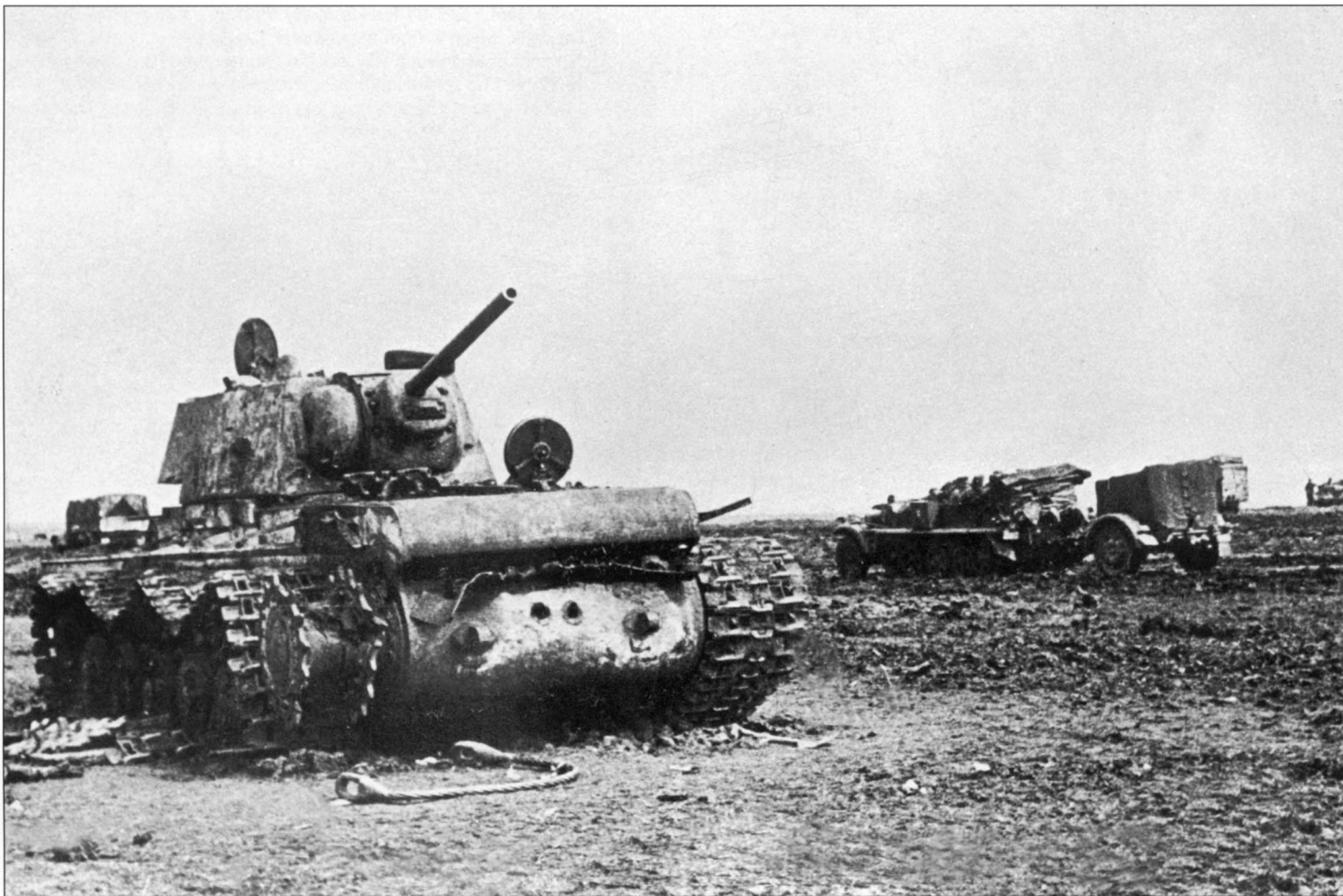
A Soviet KV-1 heavy tank demolished by German 8.8cm rounds during the spring battles. Two of the hits received by the tank are clearly visible on the rear plate of the hull. There are three other hits visible, including one on the side of the turret and two near the gun mantlet.
