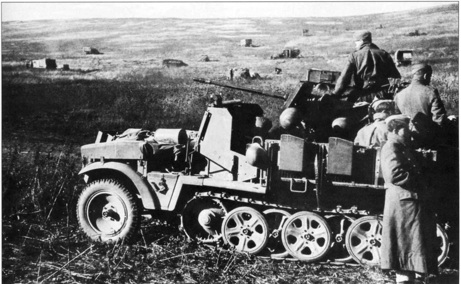
A Sd.Kfz. 10/4 with a partially armored cab and armored shield in front of the engine guards a unit's assembly area on the eastern Ukrainian steppes in the early spring of 1942. Note the binocular-type telescope installed in the driver position — a very rare piece of equipment for such vehicles, especially in this location.
