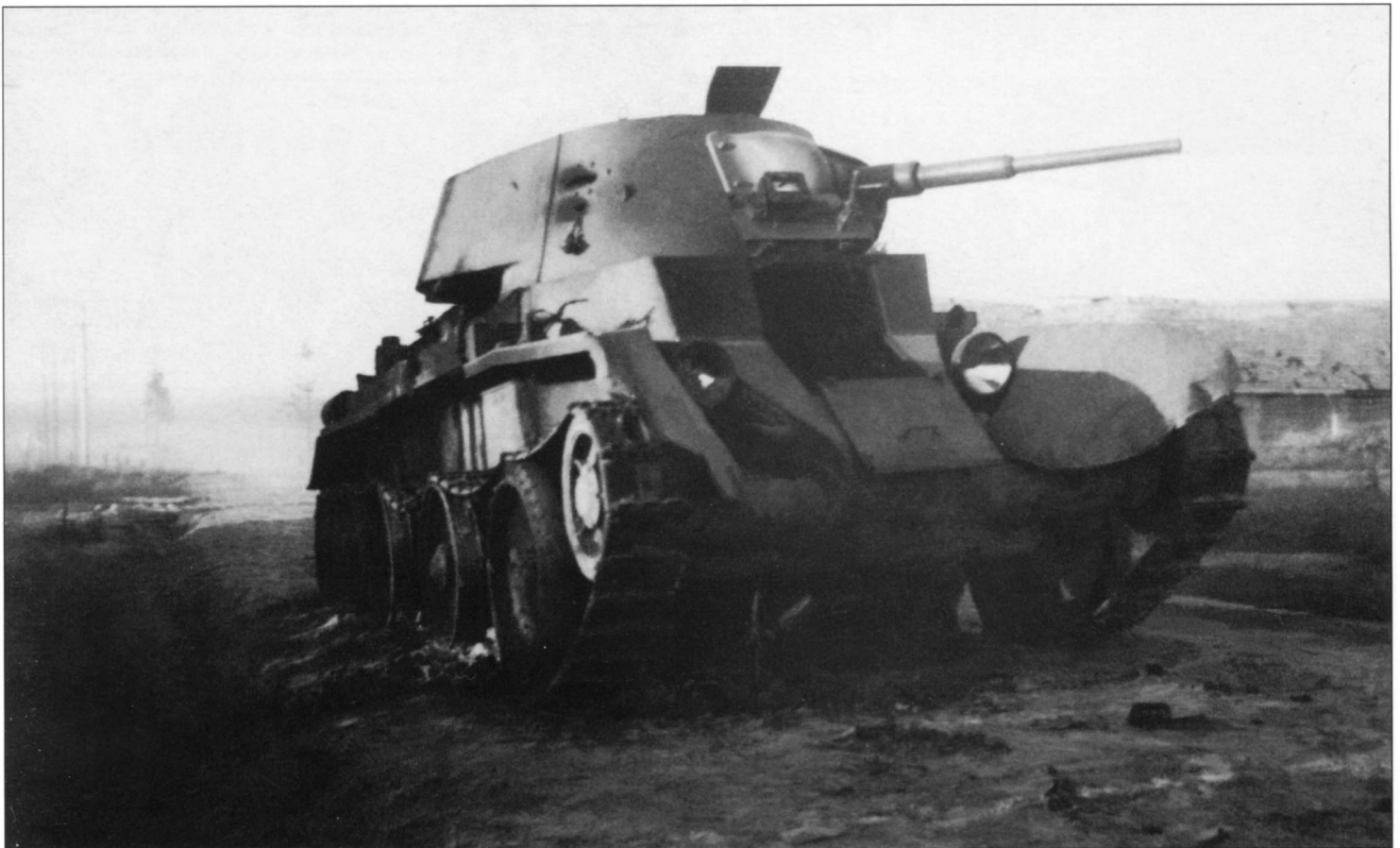
Another BT-7 abandoned on a road in a village. This tank was hit hard during a duel and was destroyed mainly by internal fire. Note the areas on the turret that have been blackened from smoke. The crew of this tank was probably lucky and escaped, a conclusion drawn from the open driver's hatch.
