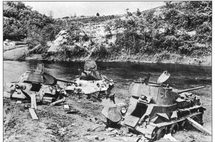
A similar situation, but this time the Soviet tank crews are in trouble. The vehicles crossed the river without much difficulty, but the muddy bank was too soft for them, especially the T-34 at the left. Both T-34 tanks are the 1941 model series, without ventilation on the turret hatch, but with thicker armor on the front of the turret.
