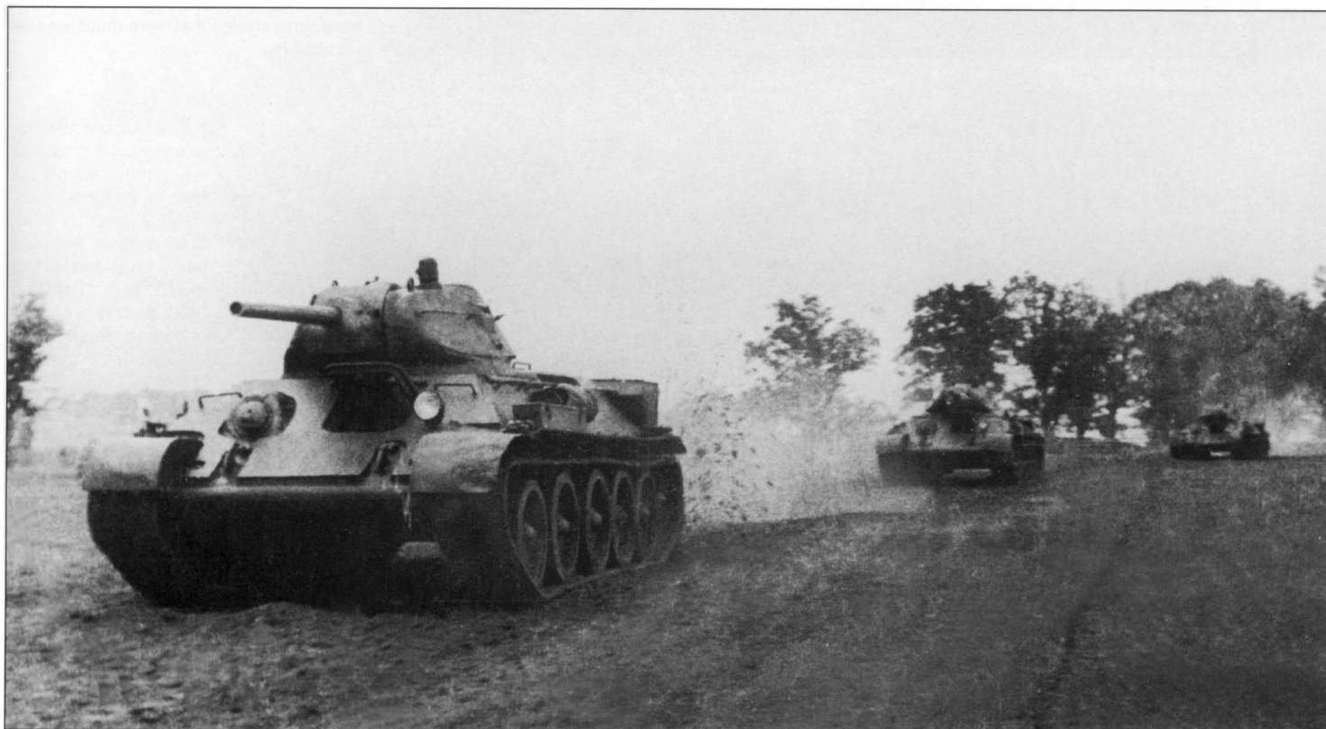
Another shot of T-34s from the same unit shows more T-34 Model 1942s produced by Plant No. 112. The lead tank has appliqué armor (about 30mm [1.25 inches] thick) welded onto the glacis front. Two factories made this modification: Plant No. 27, which produced such armor plates in 6 pieces for glacis and another for the turret, and Plant No. 112, which produced these additional plates in one piece on the glacis only.
