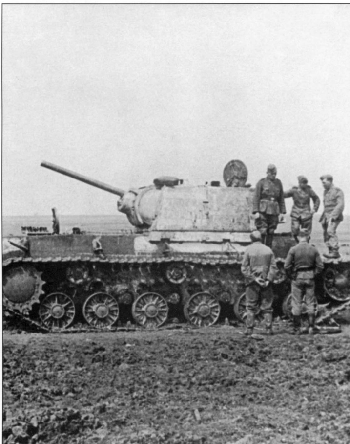
A Soviet KV-1 heavy tank demolished by German 8.8cm rounds during the spring battles. Two of the hits received by the tank are clearly visible on the rear plate of the hull. There are three other hits visible, including one on the side of the turret and two near the gun mantlet.
